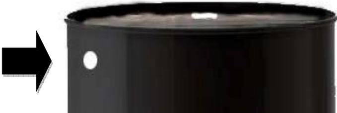
Drill a hole near the top in the side of the barrel with a  $1\frac{7}{8}$  inch hole saw for the top of the overflow.
