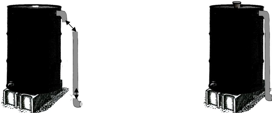
Place the flower pot with screening in the top hole. It should fit tightly but be removable for cleaning out debris.
