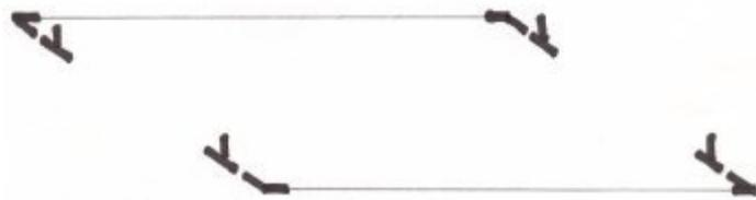
Connect two 8" pipes (one fitting at a time) between the Tees on each side of the base.
