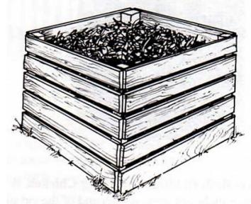
The wooden bin is easy to build. It does require more time, skill and tools than the mound or wire mesh bin and it is also more expensive than the mound or mesh bin.
